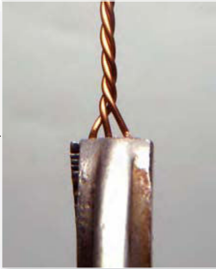
Fig. 1: Three lengths of enamelled copper wire are twisted together to form one composite 'wire' to form the balun.
